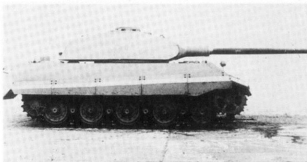
Tiger II, Prototype Fgst. Nr. VI (Chassis No. VI) with the turret produced for the Tiger P2 was accepted by the Waffenamt in November 1943. The three prototypes had the monobloc (single piece)
