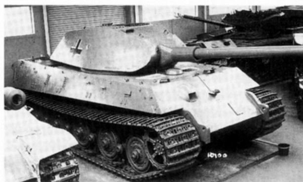
Bovington Museum has Fgst.Nr. V2 on display. As a test vehicle it has had the single link track Zg 75/800/152 fitted. This track was introduced in early 1945. The 18-tooth
